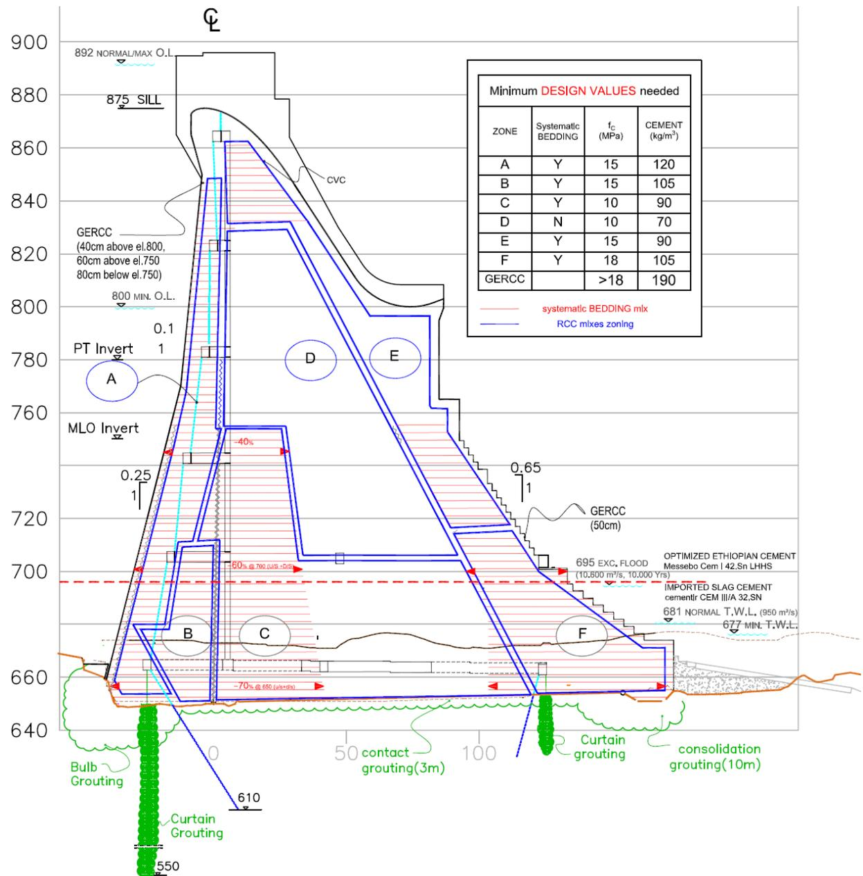
Fig. 2 Dam – Main Section with RCC Zoning
