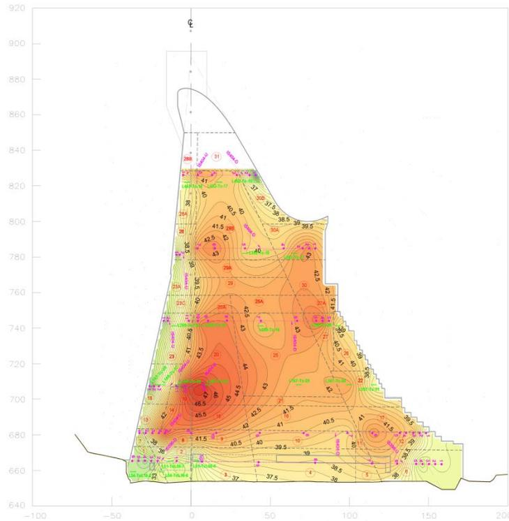
Fig.8 – Temperatures recently measured in the dam body
