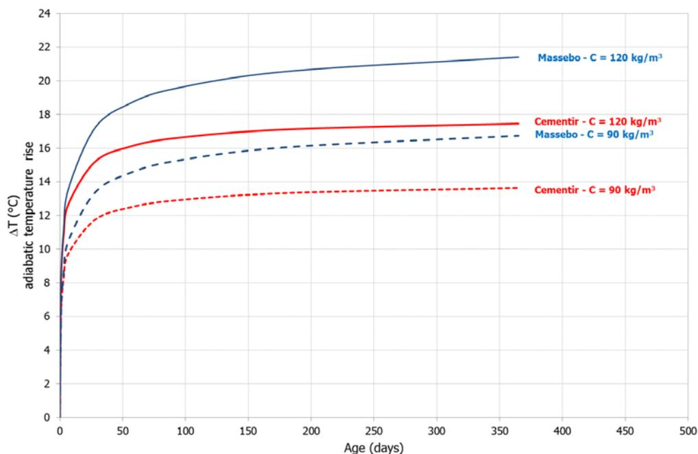
Fig.3 - Adiabatic temperature rise with Cementir and Massebo
