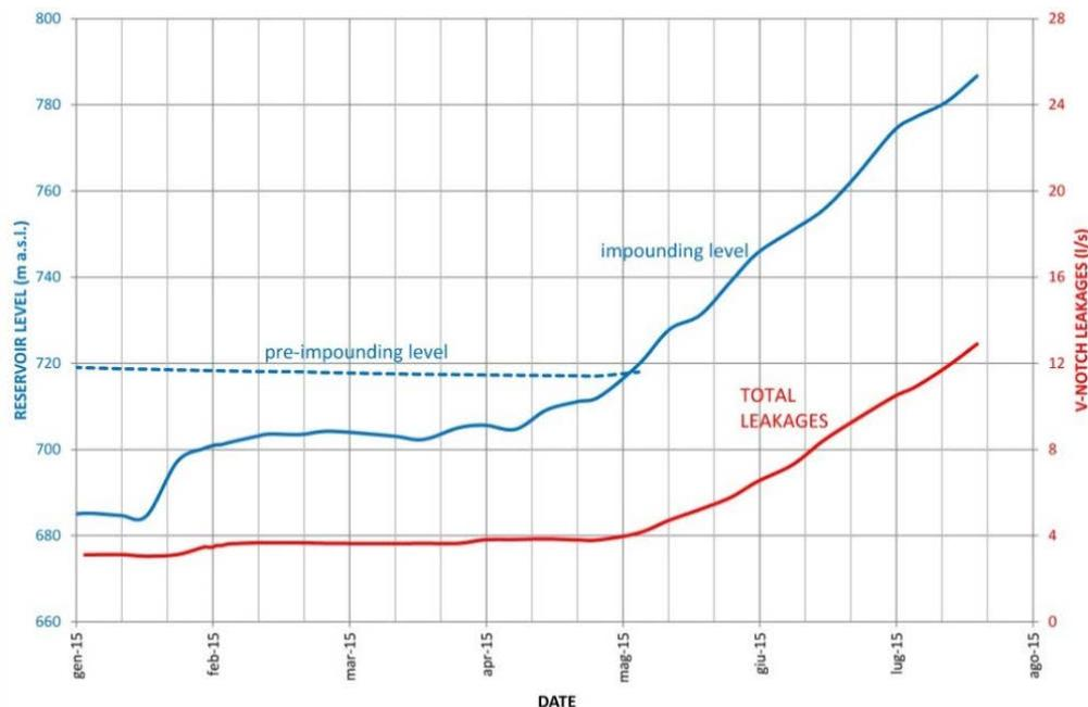
Fig. 7 - Overall leakages VS impounding level
