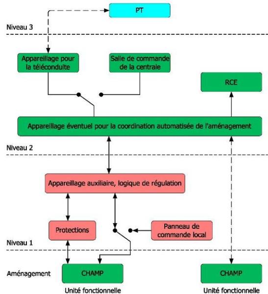
Figure 9 - configuration for the implementation of the control centres at the various levels
