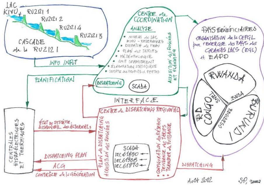
Figure 5 – RLDC, CCC, Ruzizi HPPs and GLE grid interfaces
