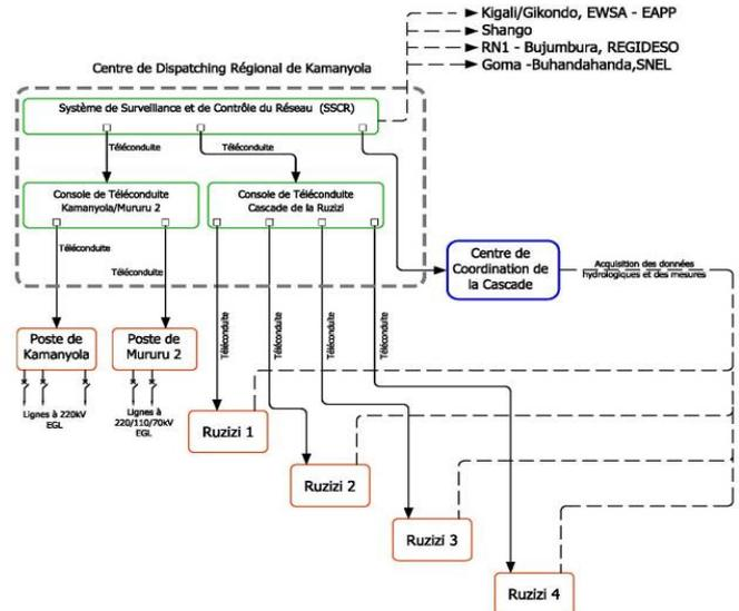
Figure 7 - conceptual scheme for telecontrol and data exchange among network, RLDC and CCC
