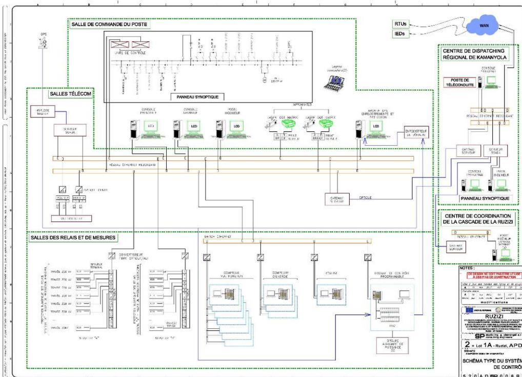
Figure 8 – Kamanyola station SCADA architecture diagram
