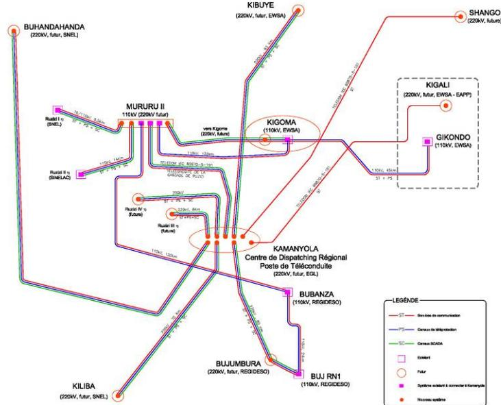
Figure 6 – Telecommunication and SCADA Diagram
