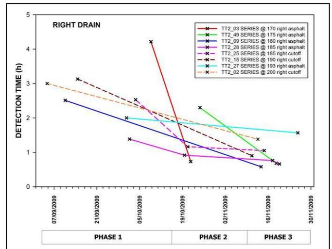
Figure 12: Second campaign decrease on the right drain of Detection times from tests performed at the same injection point.
