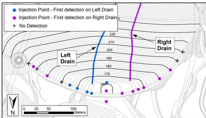
Figure 4: First test campaign injection points with indication of the drain of first response.
