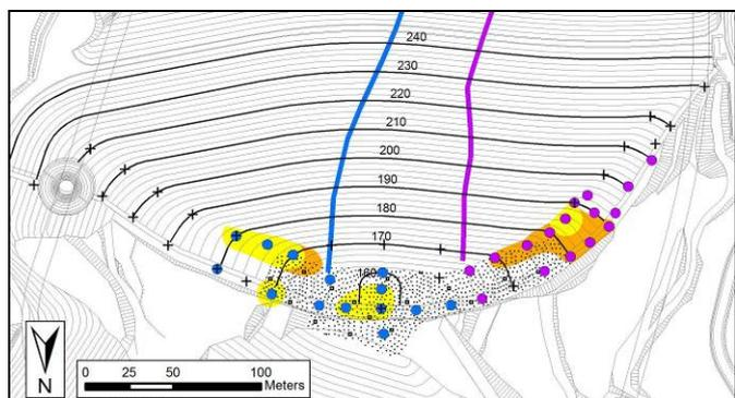
Figure 14: Second campaign Seepage zones: yellow zones observed in Phase 1, orange: extensions produced in Phase 2.
