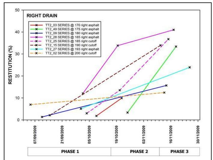
Figure 13: Second campaign Increase on the right drain of Restitutions from tests performed at the injection point.
