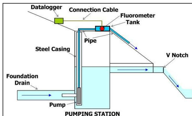
Figure 2: Detection system installed in each drain at the pumping station.
