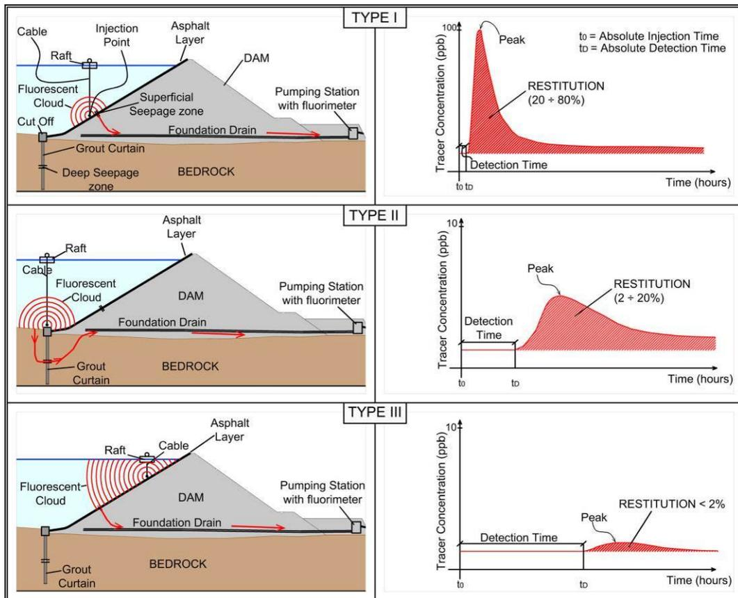
Figure 3: main types of concentration – time curves registered from the fluorimeters (right) with associated flow path of the tracer solution (left) along the dam impervious system.
